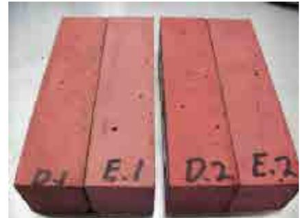
Red: Iron oxyd burgunder 3% by weight of cement (D1, E1), 5% of cement weight (D2, E2)
