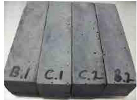
Black: Iron oxyd 3% by weight of cement (B1, C1), 5% by weight of cement (C2, B2)
