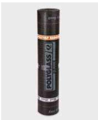
POLYVAP RADONSHIELD P-AL is a prefabricated waterproofing elastomeric-plastomeric membrane, with a distilled bitumen-based compound modified with polypropylene, reinforced with a 6/100 thickness aluminum strip bonded to reinforced glass fiber. For use as a vapor barrier and as a provisional waterproofing measure to stop water getting in temporarily, it meets the requirements of standard EN 13970.
