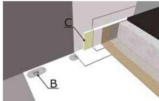
B - Spot mechanical fastening with metal stress plates and suitable screws/fasteners
