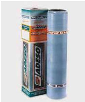
POLYVAP SA P-AL is a prefabricated double-sided self-adhesive bitumen membrane produced using ADESO technology, made up of a special selfadhesive elastomeric compound (SBS) reinforced with an aluminum foil. For use as a vapor barrier, it meets the requirements of standard EN 13970. Its use is recommended in all cases where application does not involve torching.
