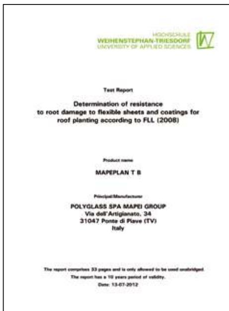
The MAPEPLAN T B waterproofing membrane is completely resistant to penetration by roots and rhizomes, as required by the strictest FLL test conducted over a period of two years, and also meets the requirements of standard EN 13948. Resistance to root penetration is one of the product's inherent properties and is not achieved with the addition of volatile substances or additives likely to wash off. The hot air welding of the overlaps and details ensure the resistance to root penetration.
