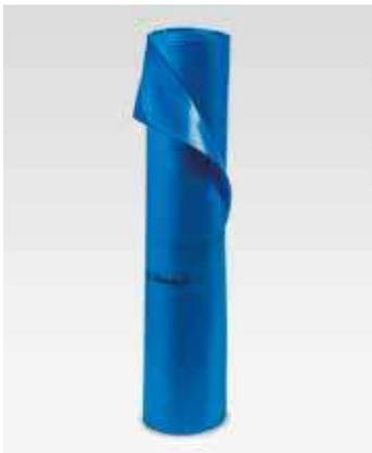
MAPEPLAN VB PE SD 220 is a synthetic sheet in polyethylene, of blue color, having a nominal thickness of 0,25 mm and  $S_d$  value of 220 m. It is used as vapor control layers and functional element for insulated roof build-ups, to be applied on the “warm side” of the thermal insulation
