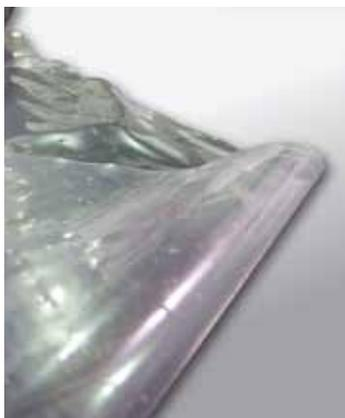
MAPEPLAN PE micro-perforated is an anti-soaking layer made from lowdensity polyethylene LDPE of transparent color, with a nominal thickness of 0.10 mm and having a micro-perforation, which makes it permeable to vapor.
