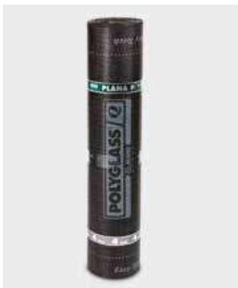
PLANA P is a prefabricated waterproofing elastomeric-plastomeric membrane, with a distilled bitumen-based compound modified with polypropylene and staple non-woven polyester fabric reinforcement. For use as a vapor barrier and as a provisional waterproofing measure to stop water getting in temporarily, it meets the requirements of standard EN 13970 and EN 13707.
